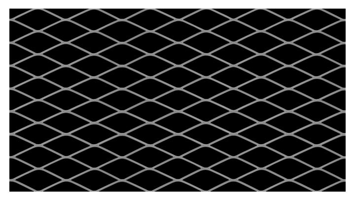
LW Pitch:30.48mmStrand Width:1.20mmSW Pitch:14.00mmThickness:0.70mmWeight:0.96 kg / m2Open Area:83%
